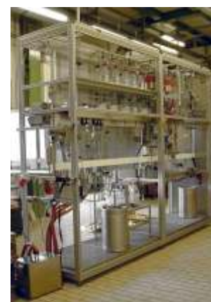
LabKit automatic polymerisation device, 25 bar, product bottling, CIP function, endoscopic camera
