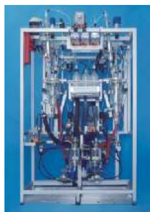
LabKit dual stage reaction system with 6 dosings, product processing and CIP function
