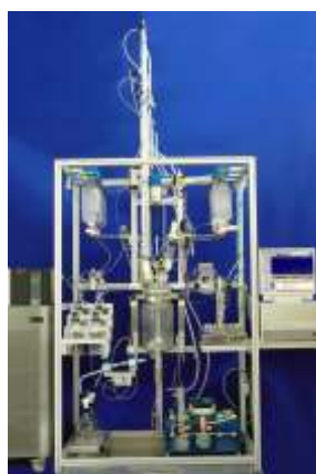
LabKit reactor system with 5 dosings, rectification with distillate weighing, phase separation and sampling
